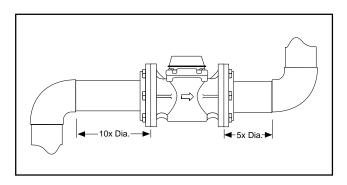
**Flanges.** Pipe flanges can be any standard 150 lb. drilling, flat or raised face. Partial or full-face gaskets may be used, but take care to insure that the gasket does not protrude into the meter due to misalignment. Adhering the gasket to the meter flange with gasket adhesive is a good practice which will aid installation.
