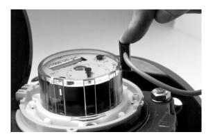
**Turbine Insert Removal.** The entire insert comes out as a unit. After relieving all pressure inside the meter, remove the four hex-head machine screws which hold the insert flange in place. Lift the flange off, rocking it if necessary to break the seal. Remove the screws which hold the insert to the flange. If necessary, the flange may now be reinstalled to allow restoration of pressure in the pipe while the insert is being repaired or replaced.
