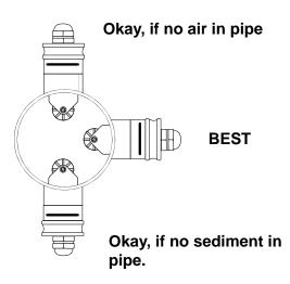
**Meter Installation.** After the meter fitting is installed in the pipeline, the meter can be installed in the fitting. Press the meter into the fitting as far as it will go. Then retain the meter in place by inserting the u-pin. This pin can be installed from either side. It is sometimes necessary to rotate the probe back and forth slightly to start the pin into the slots on the probe. Slide the pin in as far as it will go.
