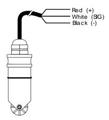
**K-factor.** If the TX80 Series meter is ordered with its fitting, the meter is factory calibrated in the fitting. A K-factor (meter factor) is indicated on the side of the fitting. This represents the actual number of pulses per gallon the meter produced during the factory flow test. This number can entered into an FT420 or FT520 flow indicator to make it read properly. If a pulse divider is being used, the K-factor is the starting point for calculating the divider number.
