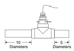
**Fitting Installation.** TX80 Series meters require special fittings. The meter fitting must first be installed in the pipeline. Straight pipe of at least ten times the diameter upstream of the meter and five diameters downstream are strongly recommended. Inadequate straight pipe, especially downstream of an elbow, change in pipe diameter, or partially-opened valves, can result in signifi-
