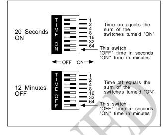
□ Set a short on-time and off-time. Then press the TEST button. The OUTPUT indicator should light and stay on for the on-time setting, and then should go out for the off-time setting. It will then repeat this cycle indefinitely. Note that the output receptacle will power up during each on-time cycle, and turn off during each off-time.
