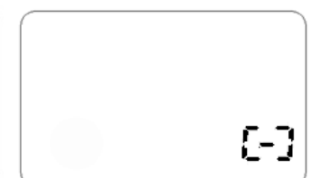
Meter Installed Backwards
