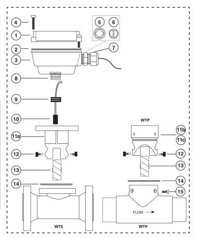
**Electronics Module Repair.** None of the electronics modules have replaceable components. Printed circuit boards must be replaced as complete units. In order to replace an entire electronics module, loosen the four retaining screws and the unit will lift free from the insert housing.
