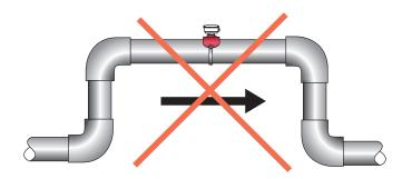
Allows air pockets to form at sensor
