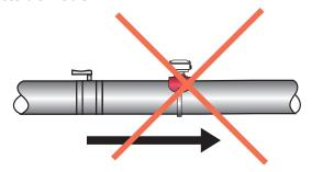
Post-valve cavitation can create air pocket
