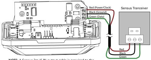
**NOTE:** A Sensus 2m (6 ft) output cable is prewired to the Seametrics product at the factory. Longer cables are optional.
