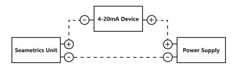
If you ever need a scaled voltage output instead of the more common scaled 4-20mA output, the milliamp signal can be changed to voltage using a resistor across the legs of the loop circuit as shown in the instruction manual.
