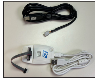
Components used for Firmware Upgrade, Programmer assembled
