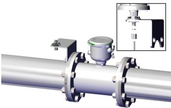
**Step 4:** Place cable thru nut. Place gasket on cable. Wire cable to Ranger. Place nut (with gasket) on mounting adapter. Tighten
