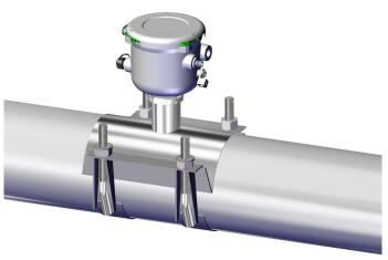
**Step 2:** Place one of the washers over the saddle bolts, on the same side of the saddle, so that they rest on top of the nuts.
