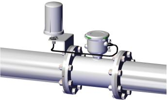
**Step 6:** Install the cable from the Ranger connector, at the bottom of the unit, to the meter connector as shown in the diagram.
