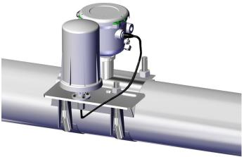
**Step 6:** Install the cable from the Ranger connector, at the bottom of the unit, to the meter connector as shown in the diagram.
