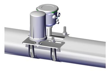
**Step 5:** Mount the Ranger to the adaptor fitting on the mounting plate.
