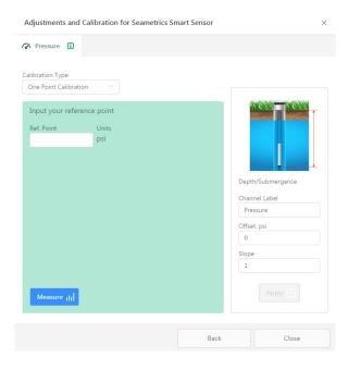
Click Apply to confirm settings and Aqua4Plus 2.0 will provide a real time reading to confirm.
