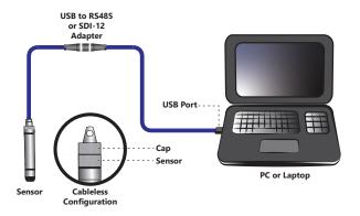
Connect the sensor to your PC using Seametrics' USB to RS485 adapter.
