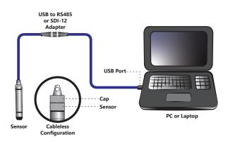
Connect the sensor to your PC using Seametrics' USB to RS485 adapter.
