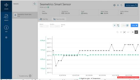
Real-time readings default to a 1 second interval for 1 minute, to adjust enter your desired settings here:
