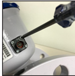
Tighten connector screws
