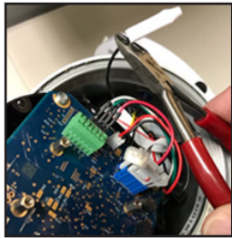
Cut the white insulator
