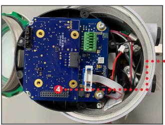
• Step 4 Gently pull on the black connector to remove the Modbus option board.
