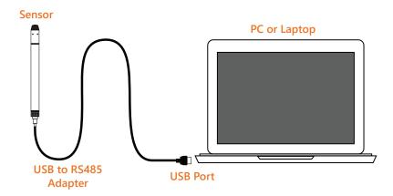
Step 3—Open Aqua4Plus, software will automatically detect your com port settings and scan for sensors
