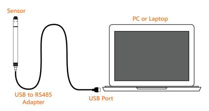
Step 3—Open Aqua4Plus 2.0, software will automatically detect your com port settings and scan for sensors
