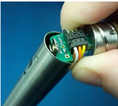
Wires tucked into slot and spring tucked into housing
