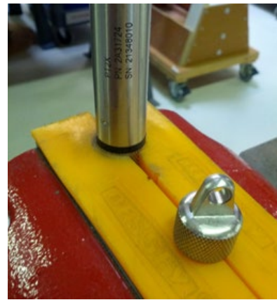
Cableless Sensor – gripping on knurled area
