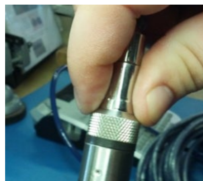
Properly completed – black ring uncompressed
