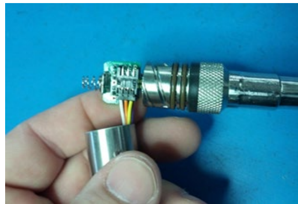
Connector properly connected
