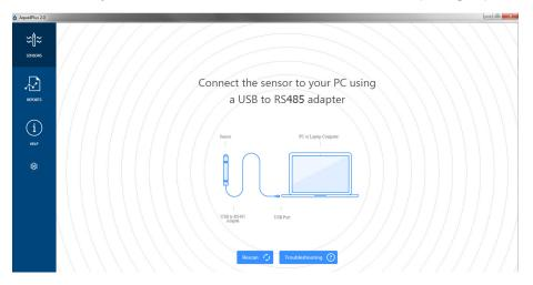
If your cable and sensor were not connected before opening Aqua4Plus simply connect and click Rescan. While scanning is active you'll see a green dot flash in the upper right corner of the program. Scanning is complete when this dot stops flashing.
