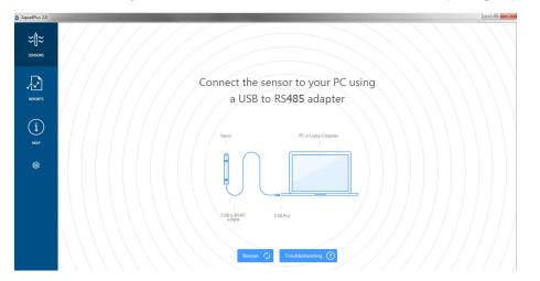
If your cable and sensor were not connected before opening Aqua4Plus 2.0 simply connect and click Rescan. While scanning is active you'll see a green dot flash in the upper right corner of the program. Scanning is complete when this dot stops flashing.
