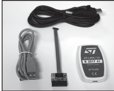
Components used for Firmware Upgrade
