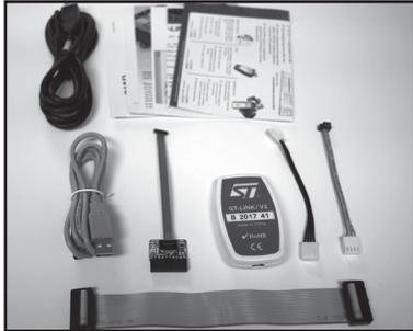
Components shipped with Firmware Upgrade Kit (Not all components included are used during firmware upgrade)
