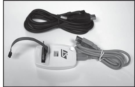
Components used for firmware upgrade (OLIMEX, Programmer & cable assembled)
