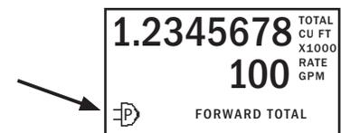
When powered by an external source, a power plug will display on any meter originally configured for external power.
