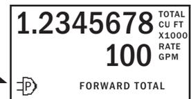
When powered by an external source, a power plug will display on any meter originally configured for external power.
