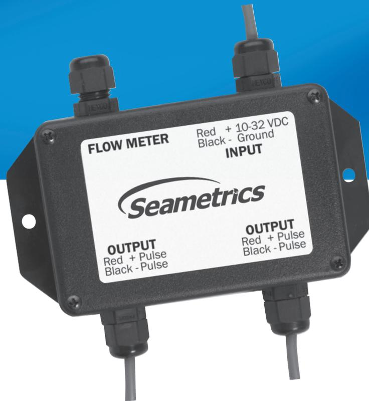
The **PS40** is a low-voltage device that allows a Seametrics flow sensor to drive multiple (up to four) pulse-responsive devices, such as solenoid-driven chemical metering pumps, counter timers, or remote totalizers. It requires an external DC power supply for operation and can provide power to a single low power Seametrics flow sensor, such as an MJE meter. It can also be used with a dry contact sensor, such as the MJR reed switch meter.
