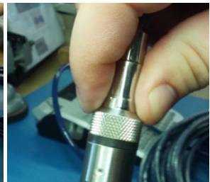
Properly completed — black ring uncompressed
