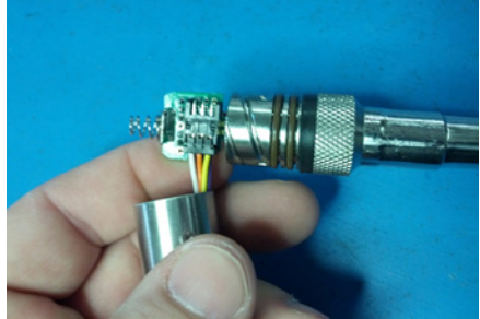
Connector connected properly
