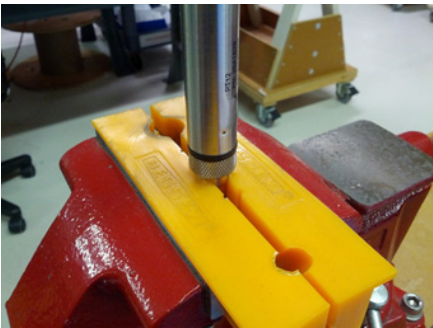
Cabled Sensor - gripping on swage
