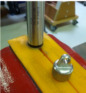
Cableless Sensor - gripping on knurled area
