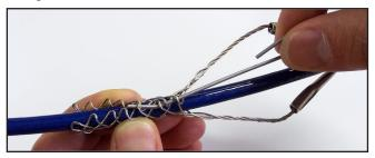
3. Continue threading until the rod is completely through the mesh.
