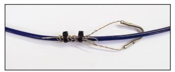
6. Attach loop to anchor hardware.
