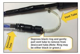
Attach vent tube to connector on the end of the bellows tube by pushing vent • tube into the opening in connector.
