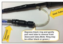
Attach vent tube to connector on the end of the bellows tube by pushing vent ٠ tube into the opening in connector.
