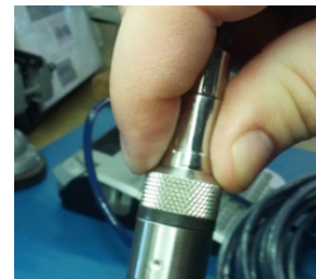
Properly completed—black ring uncompressed
