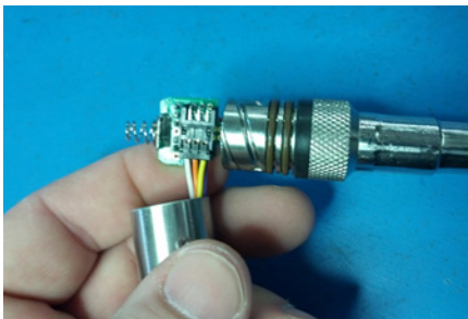
Connector connected properly
