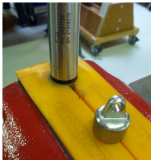
Cableless Sensor—gripping on knurled area
