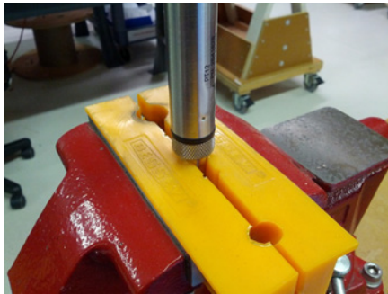
Cabled Sensor—gripping on swage
