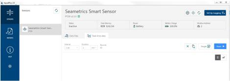
To start real-time readings click Start, readings default to table view. To switch to Real-time graphing view click the graph icon 📈
