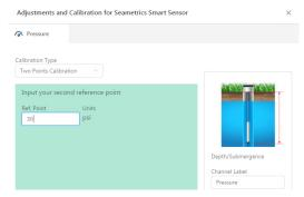
Aqua4Plus 2.0 will take 10 measurements and display the average. Watch for stability while the software is measuring to ensure an accurate calibration.
