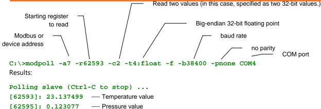
Note that the register address used is the specified address plus one. This command requested two floating point values. The program returned two16-bit registers for temperature (62593-4) and two for pressure (62595-6), interpreting both sets as 32-bit floating point values.
