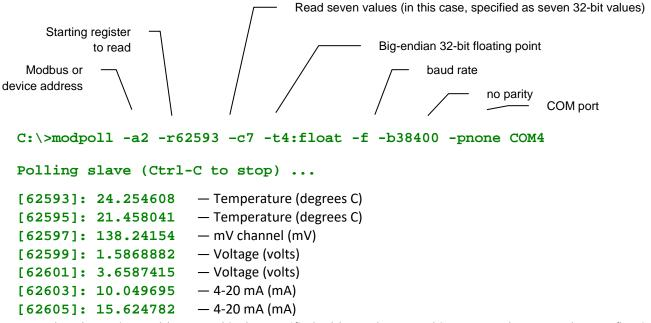
Note that the register address used is the specified address plus one. This command requested seven floating point values. The program returned two16-bit registers for each channel, interpreting each set as a 32-bit floating point value.
