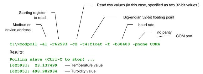
Note that the register address used is the specified address plus one. This command requested two floating point values. The program returned two16-bit registers for temperature (62593-4) and two for turbidity (62595-6), interpreting both sets as 32-bit floating point values.
