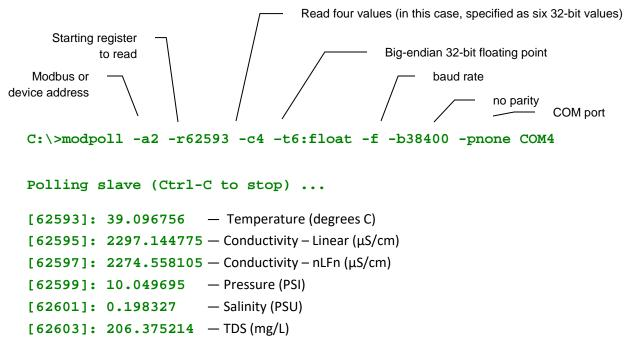
Note that the register address used is the specified address plus one. This command requested four floating point values. The program returned two16-bit registers for temperature (62593-4), and two for linear conductivity (62595-6), two for non-linear conductivity (62597-8), and two for pressure (62599-600), interpreting each set as a 32-bit floating point value.
