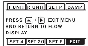
The **EXIT** tab in the MAIN MENU has a second function. If you tap five times, you will be redirected to a SUBMENU screen from which you can access additional options.
