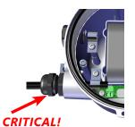
Torque cable gland sealing nut to 22 in-lbs.
