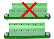
Be sure all pins align properly and that the connector has not slipped to one side.
