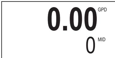
The Home screen displays total flow volume and flow rate. The four buttons below the LCD display are used to access menu screens for viewing and changing setup parameters.
