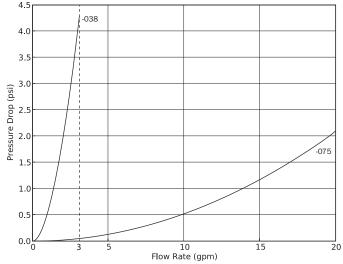
PE202-075 with 3/4" adapters. PE202-038 with 3/8" adapters.
