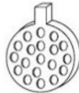
Disturbance plate (Sprenkle)
