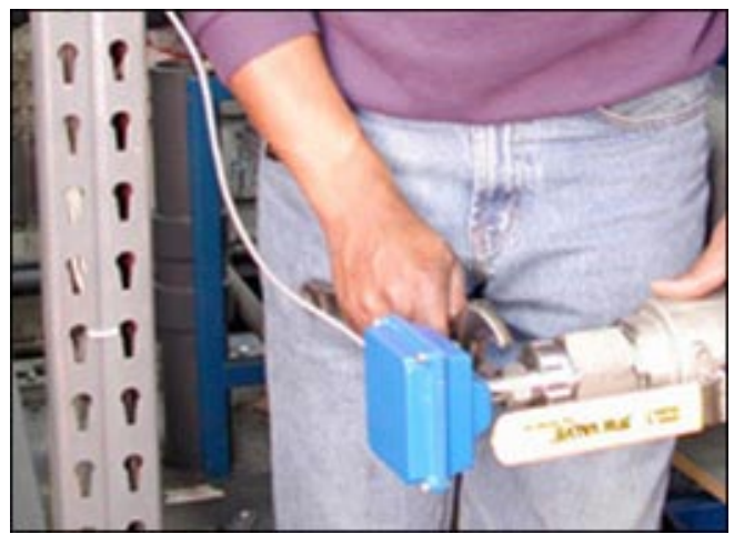
8. Adjust meter, tighten nut
