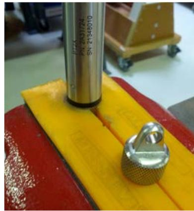
*Cableless Sensor – gripping on knurled area*
