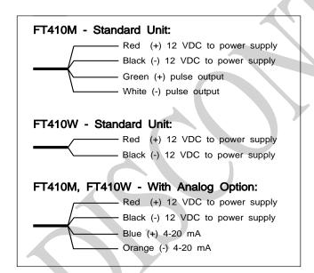
**FT410W:** This unit is pre-wired with 6 ft. of two-conductor cable for the power connections. See diagram for color coding of the leads. To complete the wiring needed for the application, remove the front clear cover, then remove the front panel to reach the terminals. Turn the front panel over, with the circuit boards still attached. Follow the connections diagram.
