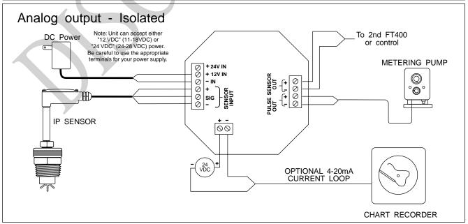
**Set 4-20 mA Span.** If the optional 4-20 mA board is installed, the prompt SET 20 mA will appear. Set this value to the flow rate, in units per minute, at which the full 20 mA output is desired. Zero flow will automatically be scaled to 4 mA.
