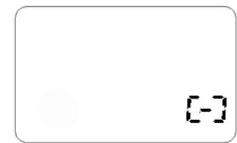
Meter Installed Backwards
