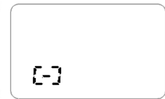
Meter Installed Backwards
