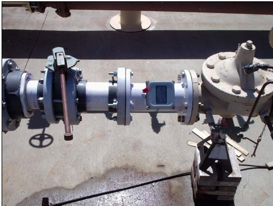
Figure 2. SeaMetrics AG 2000 test configuration for Test #3 (2 dia u/s & 0 dia d/s)
