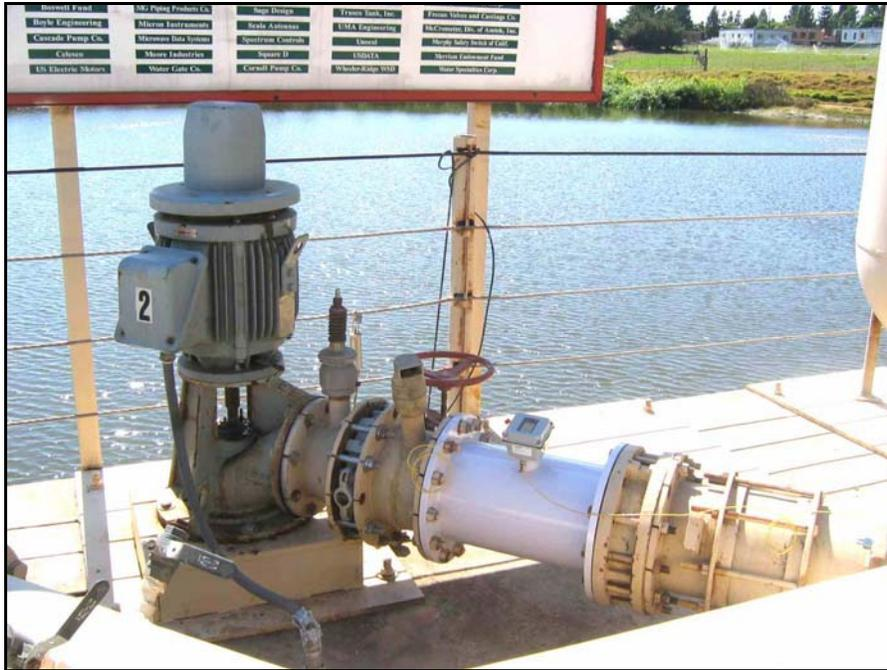
Figure 1. SeaMetrics AG2000 test condition for Test #1 (10-inch)
